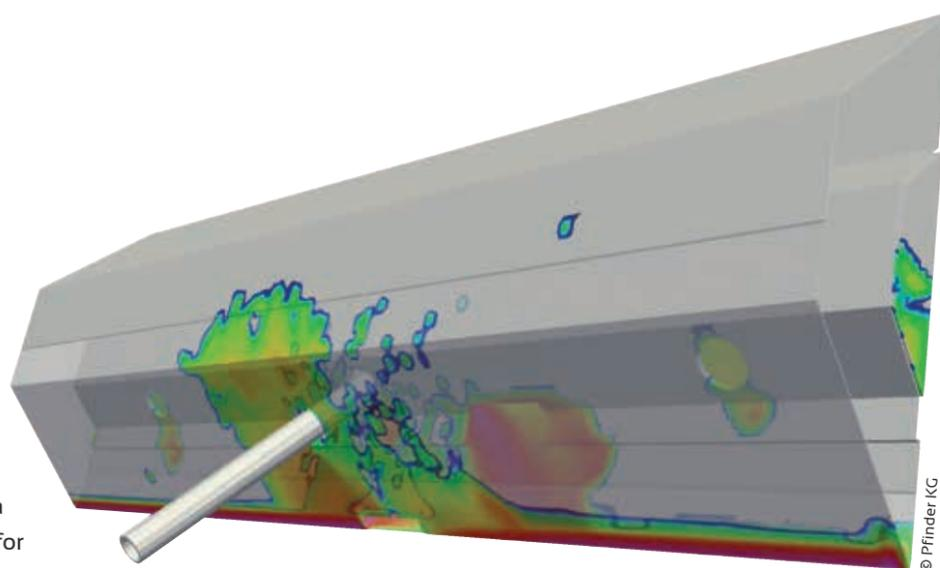
help optimize this process. Specifically, he uses OpenFOAM, a widely used software package for computational fluid dynamics, to predict how the coatings will behave when injected by a nozzle, the paths the droplets will follow through the air, and how they will form films on surfaces. These models are used to optimize the amount of fluid that needs to be sprayed for a specific application, to identify the best nozzle layout, and to ensure they are fully protective and durable.
