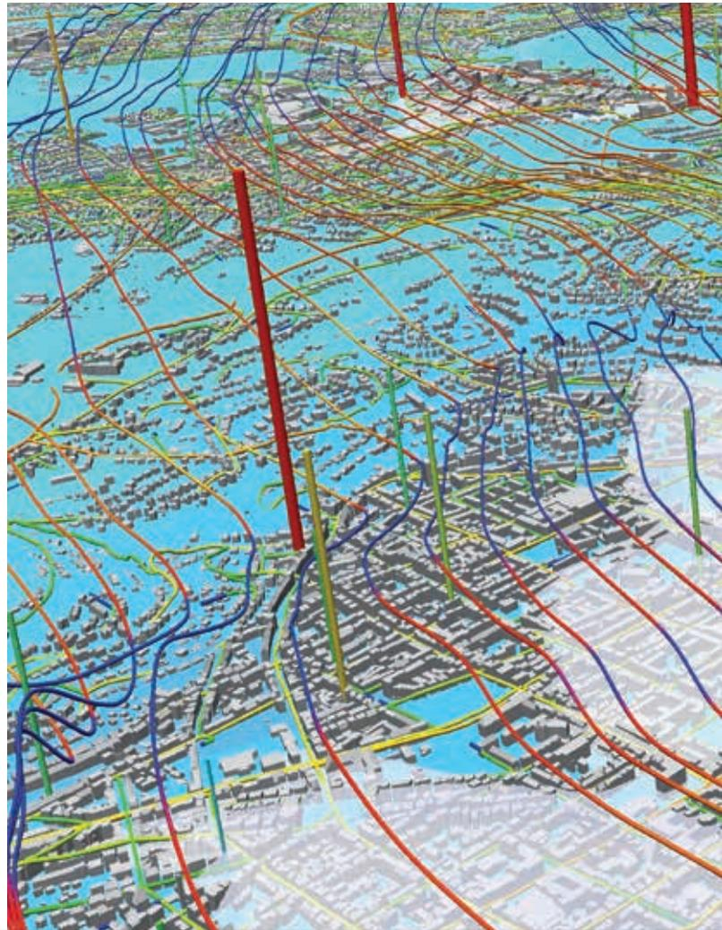
HLS developed an immersive, virtual reality-based visualization of the spread of particulate emissions in Stuttgart that makes it possible to interact with simulations at multiple scales, even down to the level of an individual street.
