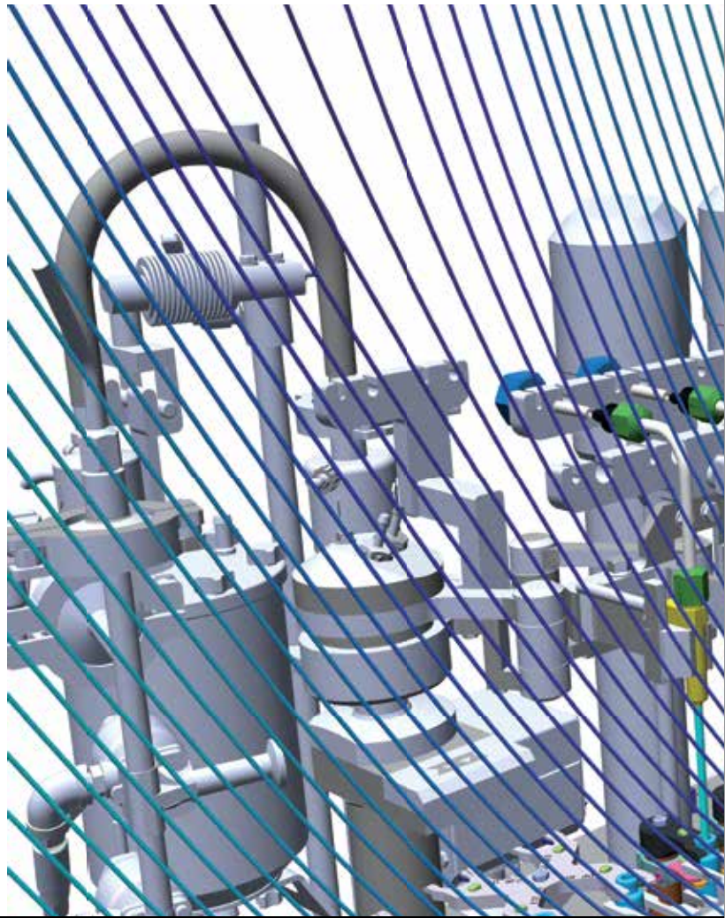
Simulation of air circulation in an automated clean room for packaging pharmaceuticals.
