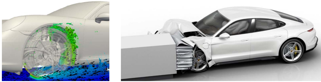
Porsche uses simulation, for example, to study water management (left) and to carry out virtual crash tests (right). Image: Porsche
