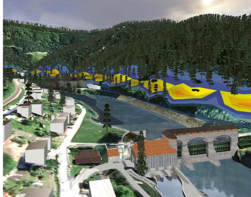
The digital twin of the Forbach facility included visualizations of data that predict construction noise.
