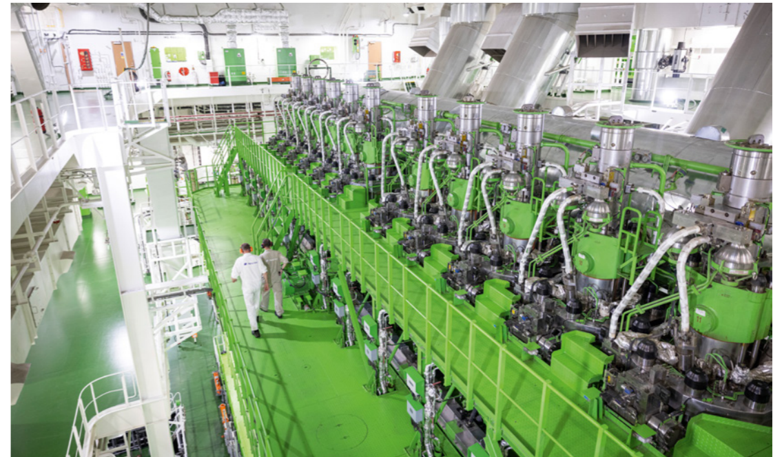
The Everllence B&W ME-GI dual-fuel two-stroke engine can run on marine fuel, liquified natural gas, biomethane, and synthetic natural gas.
