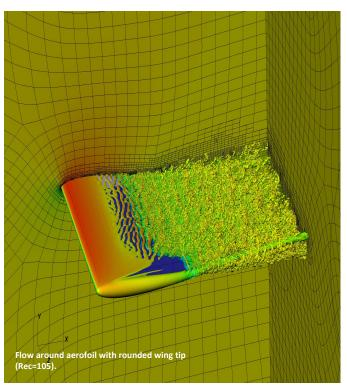
Adaptive mesh refinement is implemented, which improves computational efficiency in rototcraft off body grid by 50-70% of total cell (new implementation).
